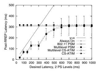
Fig. 9. Latency threshold versus observed latency using two power save levels.
