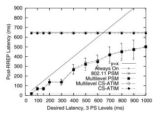
Fig. 12. Latency threshold versus observed latency using three power save levels.
