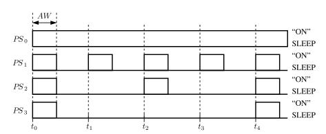
Fig. 2. Multilevel power save with 802.11 PSM [9].
