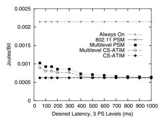
Fig. 11. Latency threshold versus energy consumption using three power save levels.
