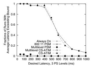
Fig. 13. Latency threshold versus observed latency using three power save levels.
